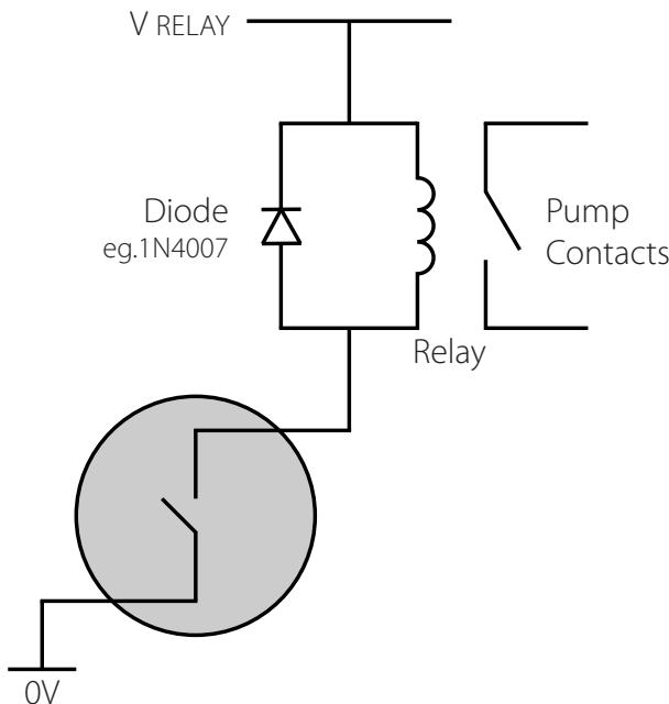
The diode **MUST** be fitted across the relay coil as shown to prevent potentially high voltages being generated by the relay coil when switched off - known as 'back EMF'. Without the diode, the voltage can rise to several hundreds of volts and destroy the electronic switch.
