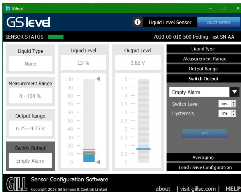
This example shows the Switch Output set to an EMPTY ALARM with a switch level of 10%. When the liquid level reaches 10% the open collector switch will activate. This may operate a pump or a valve to add fluid to the tank.
