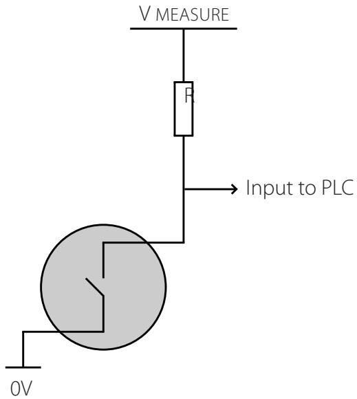
V MEASURE is selected to match the PLC measurement requirements but must not exceed the electronic switch maximum ratings. The input channel on the PLC may be an 'analogue' or 'digital' line depending upon V MEASURE. The value for R is arbitrary, a typical range being 1KΩ to 10KΩ.
