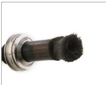
WearDetect with coarse and fine debris attracted to the sensor head face.
