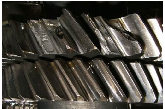
Gear tooth breakage leading to expensive repairs and loss of production
