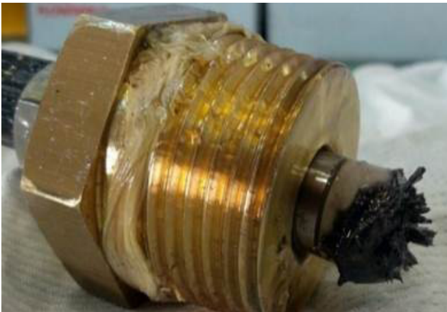
Debris build-up collected from a large speed - gearbox system.
